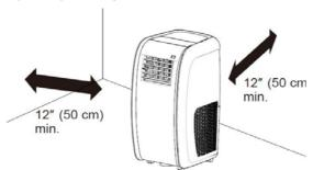
• Place the unit in an area where the temperature will not fall below 16 ℃ (61°F). The coils will be covered with frost at temperatures below 16 ℃ (61°F), and this may reduce performance.
