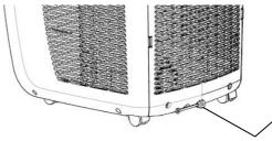
Drain plug location, a drain hose, plug and hose clips are supplied with the unit. These can be fitted to the unit when draining the tank.
