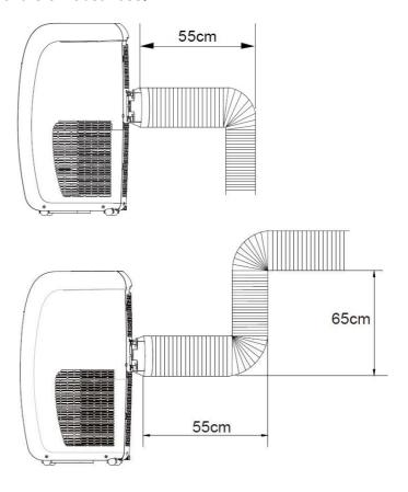
Wrong installation of the exhaust hose is shown below. If the hose is to bent, the unit will not function correctly.
